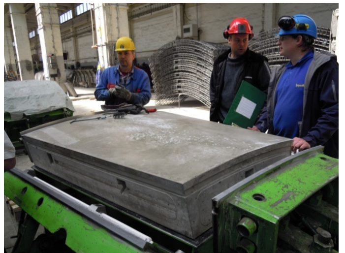
Figure 4. Production of SFRC key segment for trstiny (a – casting; b – demoulding)
