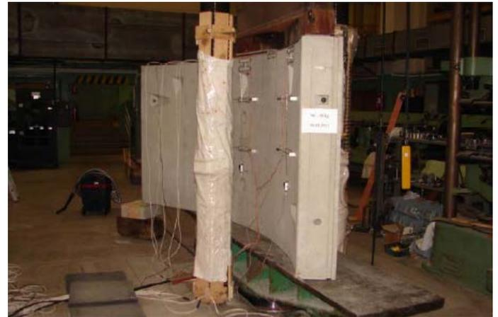
Figure 7. A segment compressed by two loads
