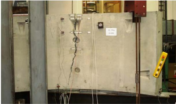
Figure 10. SFRC segment disturbed by loading by bending in the segment plane
