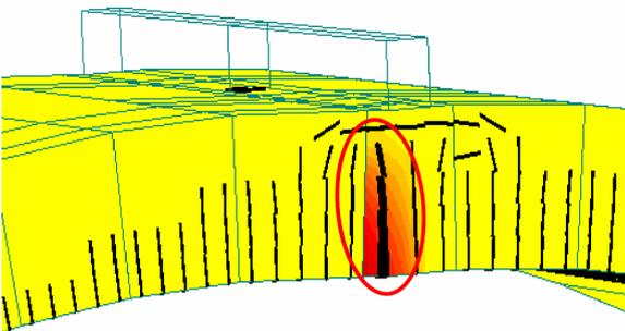
Figure 11. Comparison of crack locations from test and numerical modelling, SFRC segment loaded by bending perpendicular to segment plane
