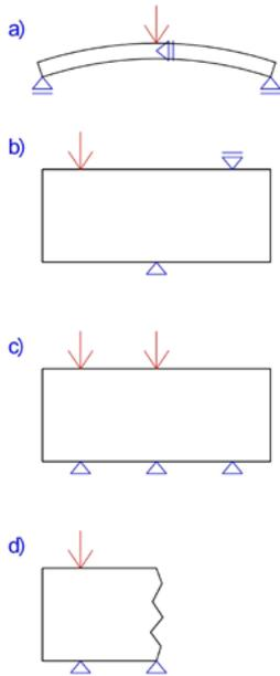
Figure 1. Conducted tests – a) segment bending perpendicularly to the segment plane, b) segment bending in the segment plane, c) unilateral pressure on the segment induced by two loads, d) unilateral pressure induced by a single load acting on remains of segments
