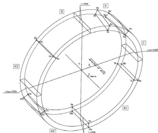
Figure 2. Geometry of segments in a lining ring
