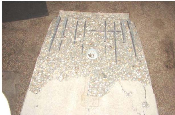
Figure 8. Delamination of traditionally reinforced concrete segments loaded by unilateral pressure
