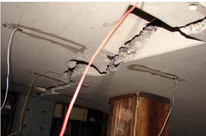
Figure 4. A segment loaded by bending perpendicular to the segment plane (underside view)
