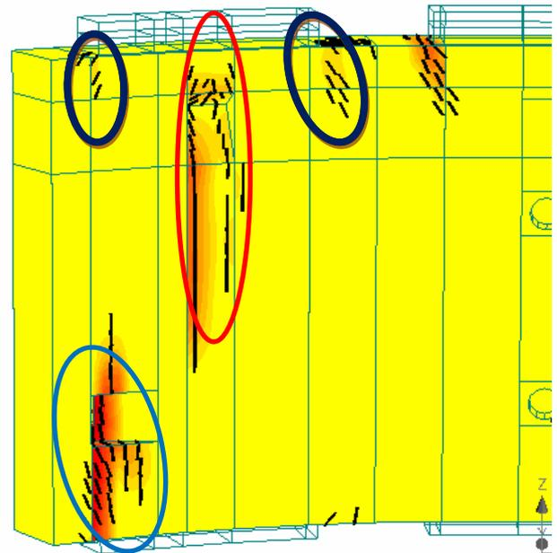
Figure 12. Comparison of crack locations from test and numerical modelling, RC segment loaded by axial compression
