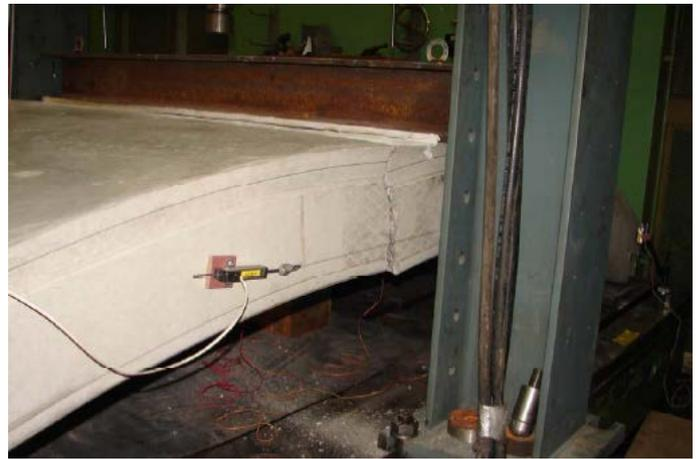
Figure 5. A segment loaded by bending perpendicular to the segment plane after becoming disturbed (side view)
