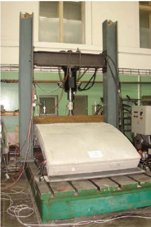
Figure 3. A segment loaded by bending perpendicular to the segment plane
