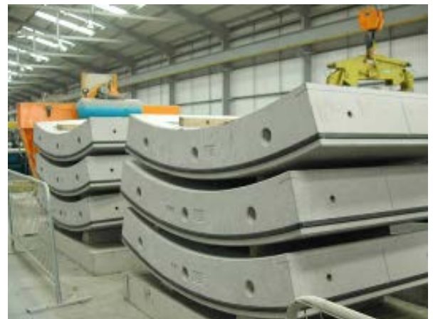
Figure 3. Storage of pre-cast steel bar reinforced concrete segments
