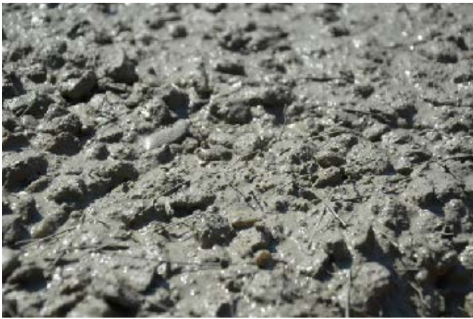
Figure 4. Fresh SFRC (the length of fibres is 60 mm)
