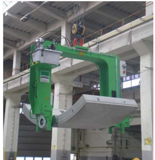
Figure 2. Segments handling during production
