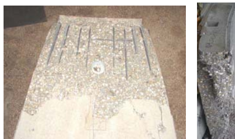
Fig. 7 Comparison of damaged key segments after reaching their capacity: a) RC key segment, b) SFRC key segment
