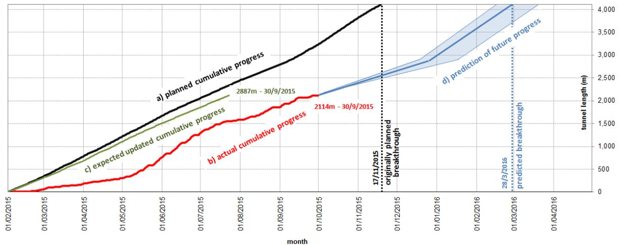
**Figure 1.** Construction schedule: a) black – originally planned excavation progress based on expected excavation classes; b) red - actual excavation progress shown till the end of September 2015; c) green – expected updated excavation progress based on actual excavation classes and advance rate as per bid; d) blue – probabilistic prediction of future excavation progress based on previous excavation data.
