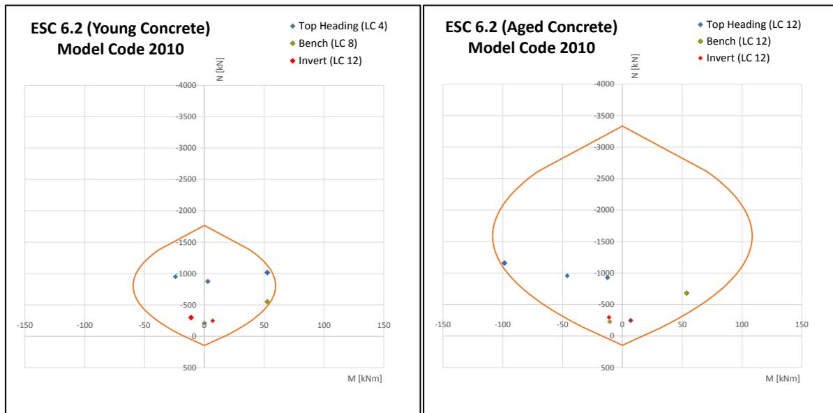
**Figure 8.** Assessment of load bearing capacity with positive effect of fibres (ESC 6.2)
