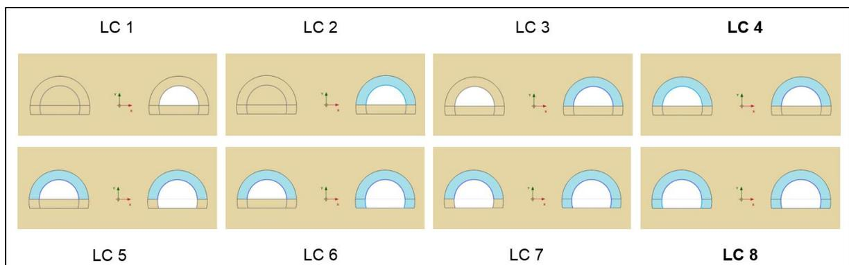
**Figure 3.** Load case schematics for the excavation support class 5.1
