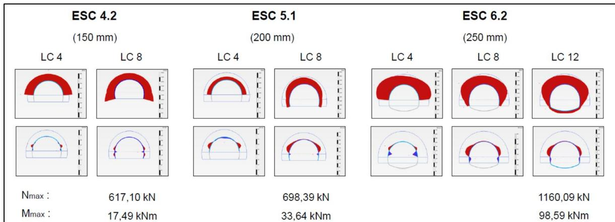
**Figure 4.** Calculated internal forces in the primary lining for the particular load cases (LC)
