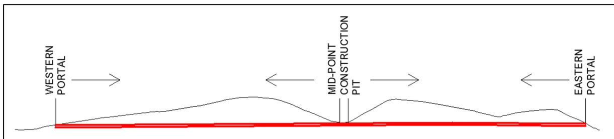
**Figure 1.** Construction sequence schematic shown in longitudinal section
