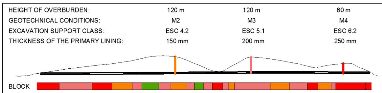
**Figure 2.** Locations and basic parameters of analysed FRSC sections
