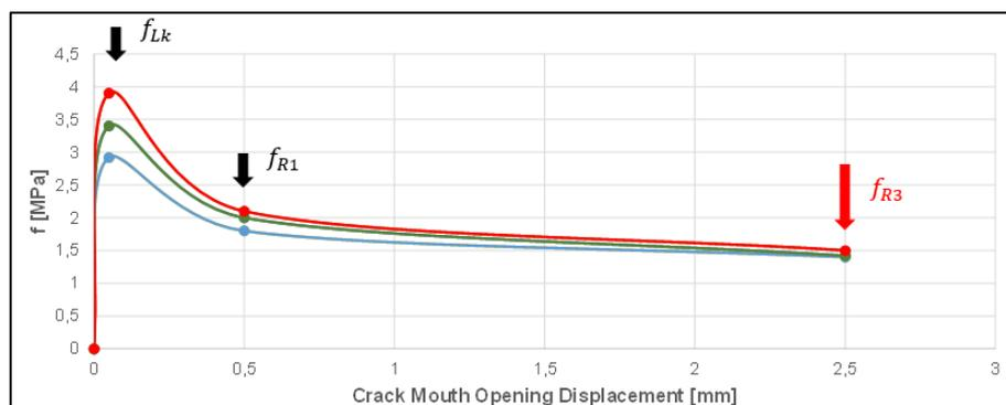
**Figure 5.** Results of three point load test (flexural tensile strength vs crack mouth opening)
