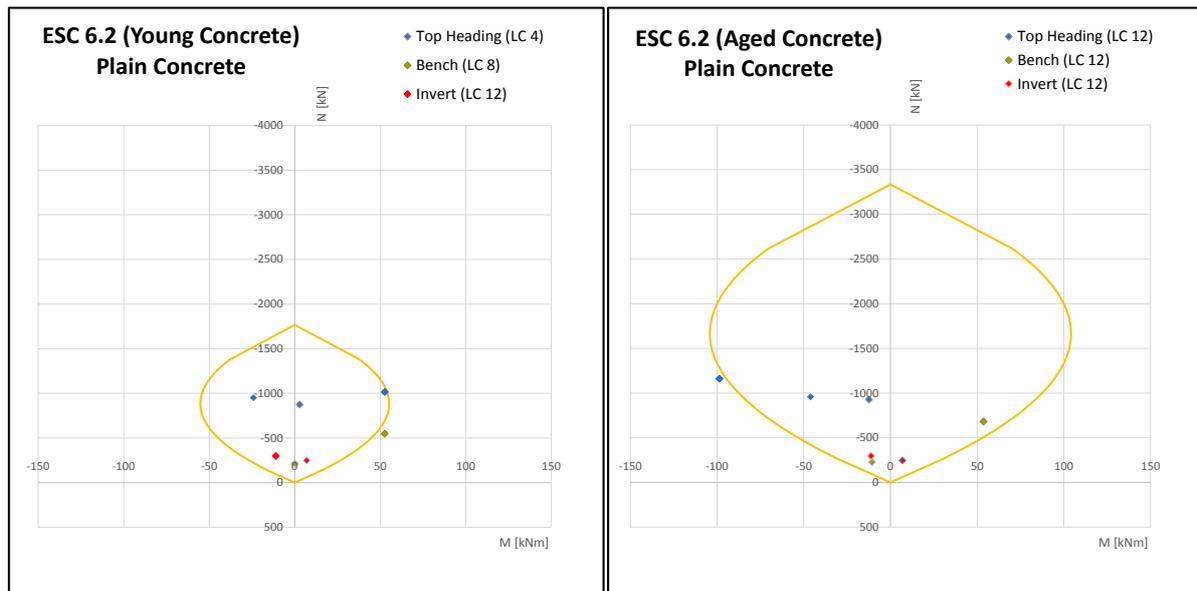
**Figure 7.** Assessment of load bearing capacity **without** positive effect of fibres (ESC 6.2)
