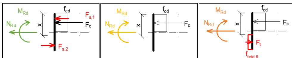
**Figure 6.** Principle for calculation of load-bearing capacity (wire mesh, plain concrete and fibre reinforced concrete)
