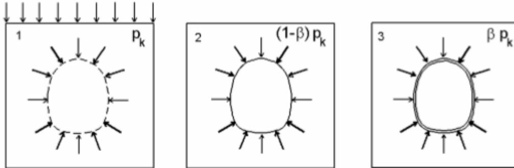
Figure 4: Schematic representation of the  $\beta$ -method, [5]
