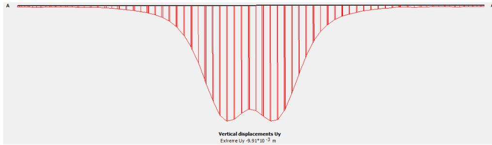
Figure 12: Surface settlement profile of cross section A-A\*
