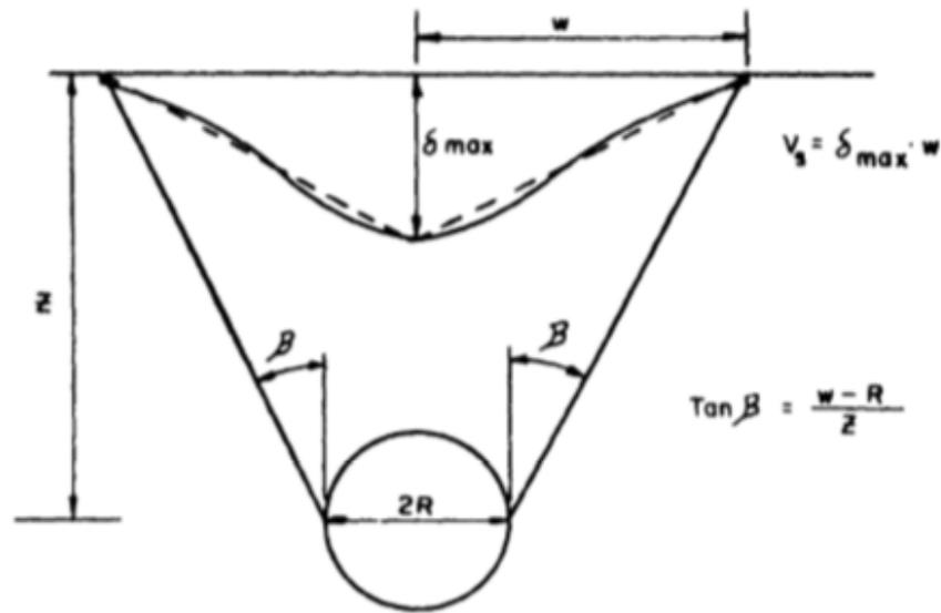
Figure 2: Relation of  $\beta$  to through width [3]
