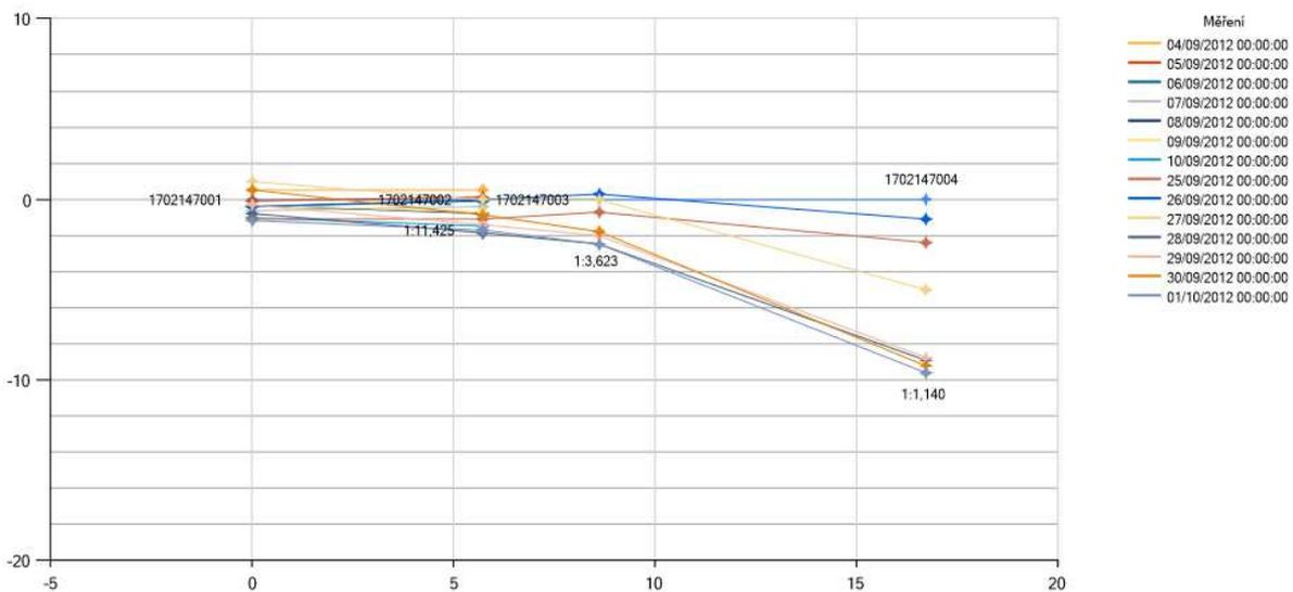
Figure 13: Cross section of ground surface settlement at the position of 15.3 km [7]
