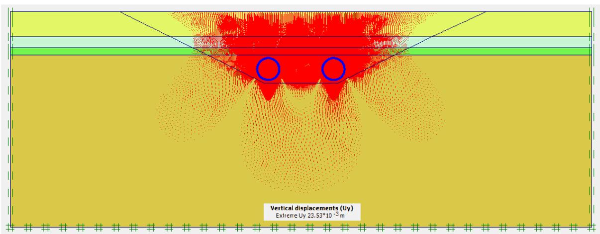
Figure 7: Vertical displacement (arrows) – variant I
