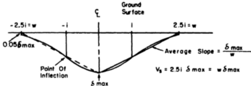
Figure 3: Width of the settlement trough, [3]
