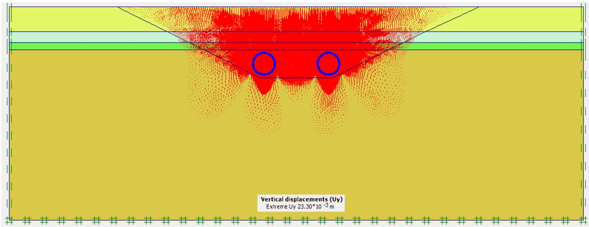
Figure 8: Vertical displacement (arrows) – variant II
