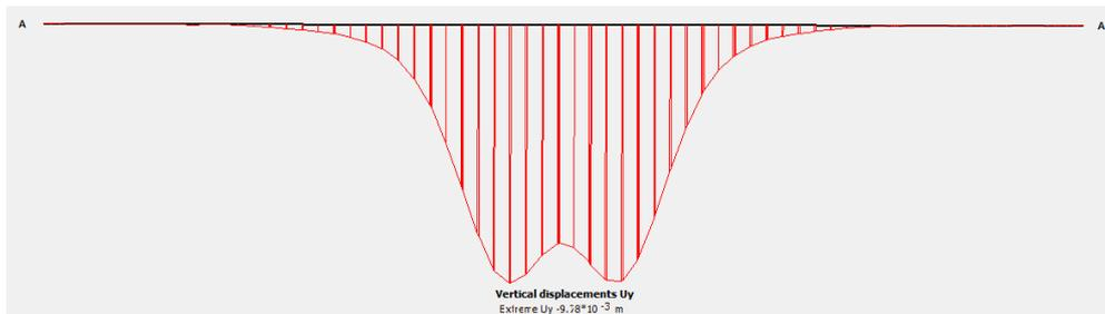
Figure 112: Surface settlement profile of cross section A-A\* - variant I
