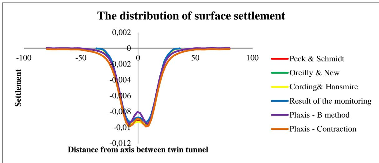
Figure 14: Surface settlement – comparison of twin tunnel results
