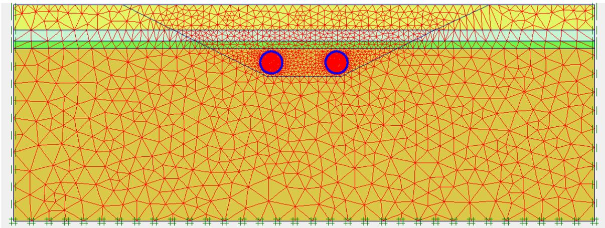
Figure 1: Generated mesh for single tunnel
