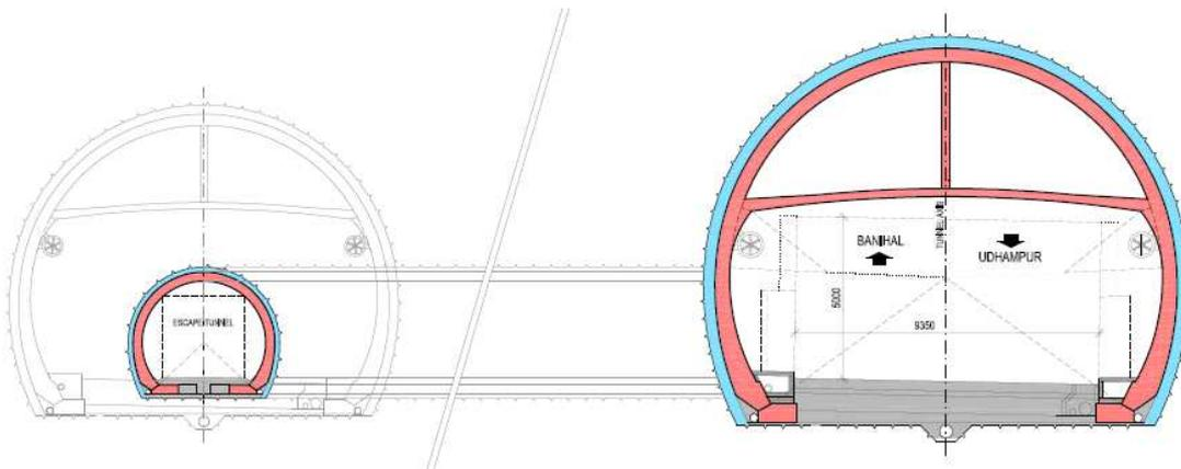
Figure 2 Tunnel cross section (DPR) and safety concept with foreseen possibility of future extension to a double lane, unidirectional tunnel
