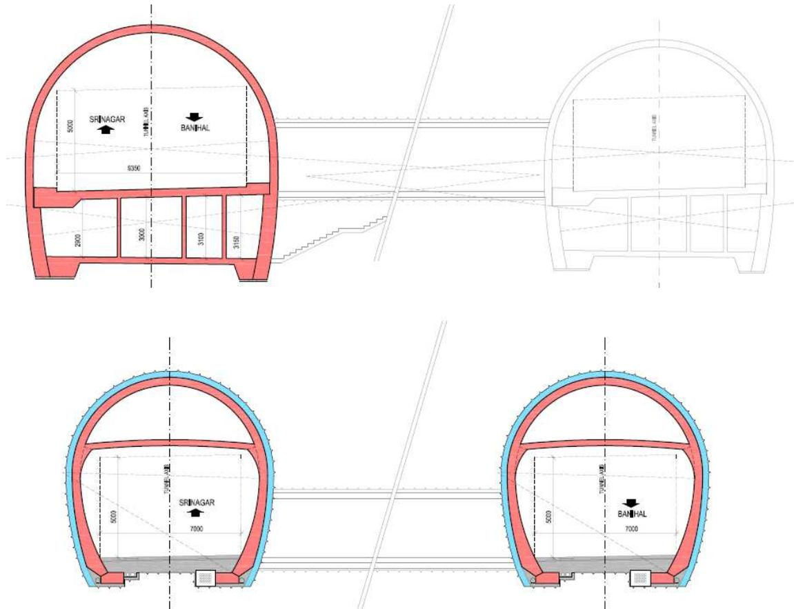
Figure 4 Development of the concept solutions for Pir Panjal road tunnel (above DPR solution, below concessionaire solution)
