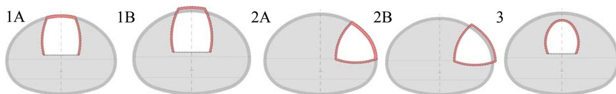
Fig. 4 Positions and geometries of pilot adits and their examples (1 - PCRR 513, PCRR 514; 2 – Královo Pole tunnel, Brno; 3 – Mrázovka, Královská Obora, Prackovice tunnels)
