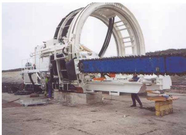
Figure 4. Prevault/Perforex method and machine
