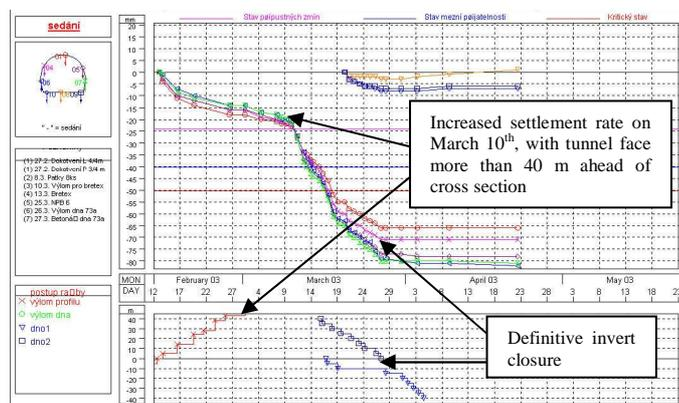
Figure 7. Monitoring of tunnel deformations
