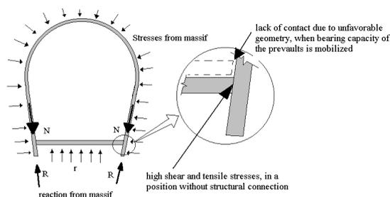
Figure 5. Bottom slab function
