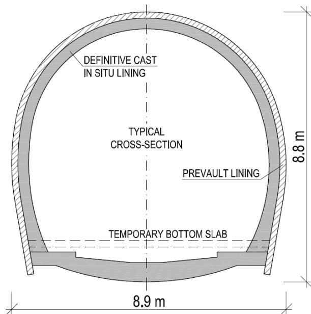
Figure 3. Tunnel cross section – primary and final lining
