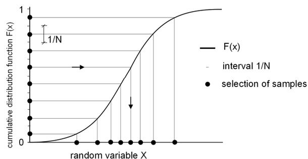
Figure 1. The principle of the LHS-median sampling
