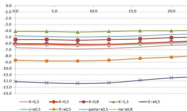
Figure 9. Vertical deformation of the surface along the tunnel axis [mm], Red line – initial parameters, max.  $E \cdot \frac{1}{2}$ , min- settlement  $K_0=1.3$
