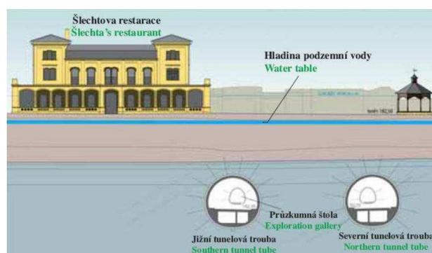
Figure 4. The Blanka tunnel cross section
