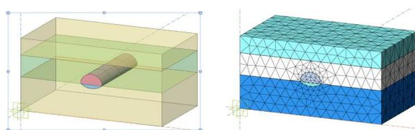
Figure 7. 3D model of the Petřiny station in Midas GTS
