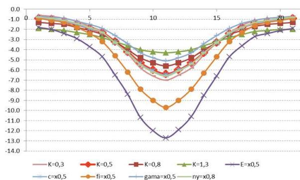
Figure 8. Vertical deformation of the surface perpendicular to the tunnel axis [mm], Red line – initial parameters, max.  $E * \frac{1}{2}$ , min- settlement  $K_0=1.3$
