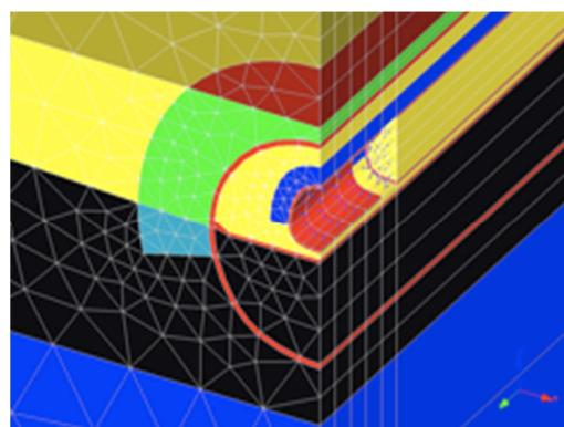
Figure 5. 3D model of the Špejchar – Pelc-Tyrolka tunnel (detail of the exploratory drift)
