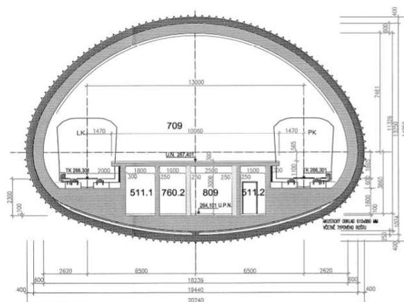
Figure 6. Cross-section of the Petřiny station
